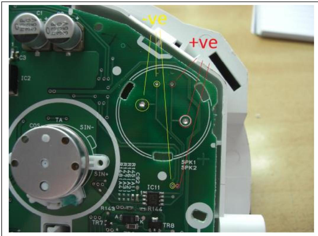
Speaker is controlled by TDA7052A/AT (1 W BTL mono audio amplifier with DC volume control) for your reference.
