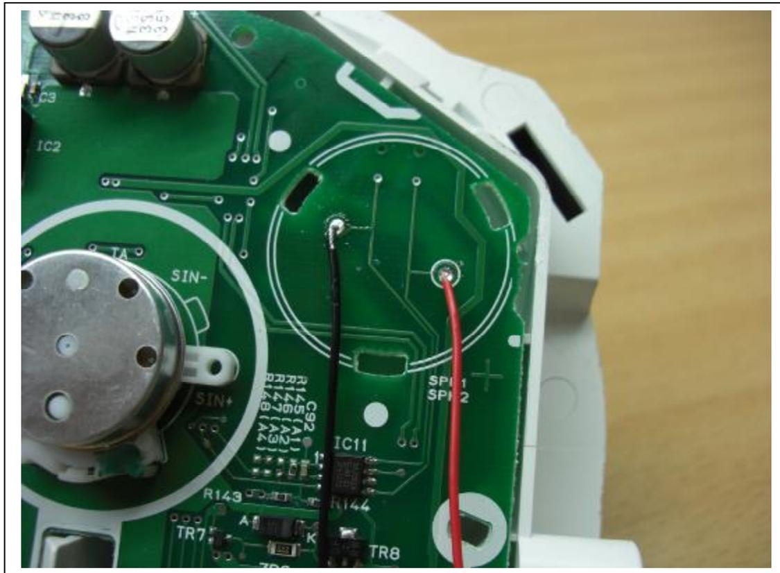
If you can't find a speaker that fits internally within the space of the one you removed, you can pass the wires out the back of the vents and place it where you see fit.
