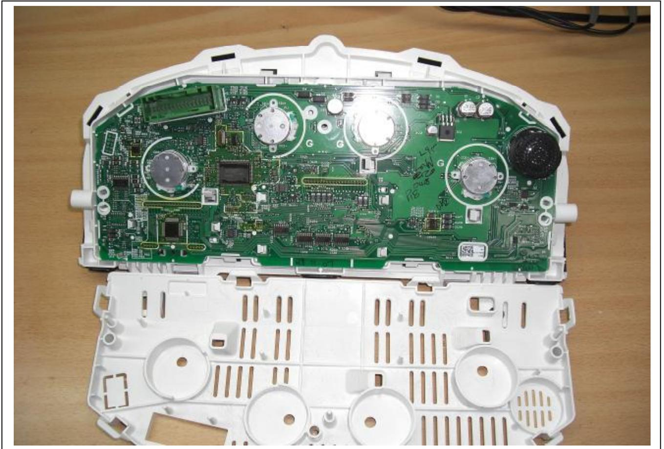
Locate and de-solder the loudspeaker with its cover still on. Bit tricky due to the plastic clips.
